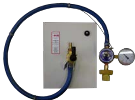
HIGH SIDE GAS BOARD
