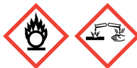
Flame over circle Corrosion
